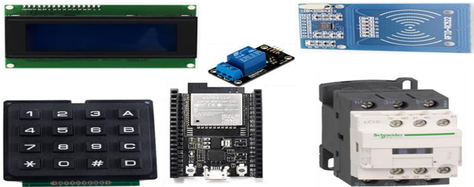
Figure 6: Hardware components of the EV charging node
