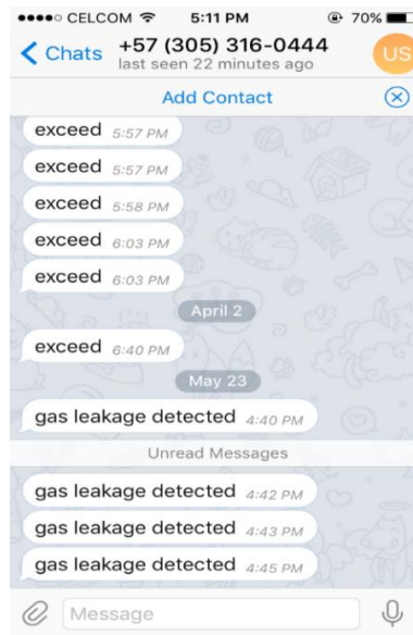
Fig. 11. Image shows that when the gas detected exceeded the set value, the user will get a telegram message.
