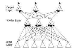
Fig.4. Architecture of Back Propagation Neural Network
