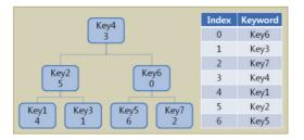
Fig. 5 B-Tree Structure for High-Speed Preprocessing.
