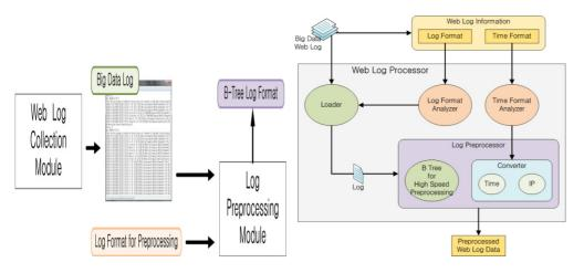
Fig. 3 High-Speed Preprocessing of Big Data Mobile Web Log.
