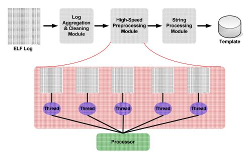
Fig. 6 Thread-based Parallel Processing for Preprocessing of Mobile Web Log.
