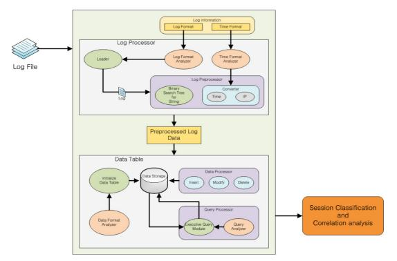
Fig. 7 Big Data Mobile Web Log Preprocessing for Detecting Attacks.
