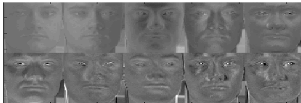
Fig 1. Leading 10 Eigenfaces trained from 44 images of a sample subject of the PIE illumination face database.
