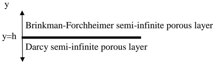
**Fig. 4.** Representative sketch of coupled parallel flow
