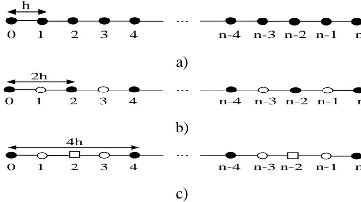
**Figure 1** a), b) and c) show distribution of uniform solid node points for the full-, half- and quarter-sweep cases respectively
