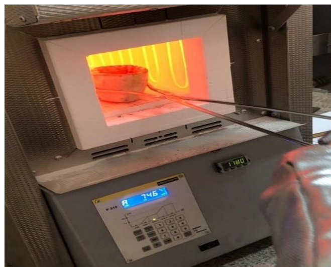
Fig. 3. Preparing the shape memory alloy using an electric furnace
